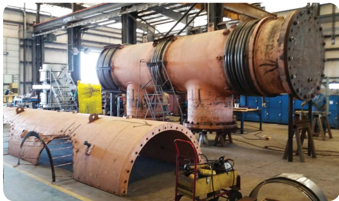
Disassembly of a Wrapper Crossover
