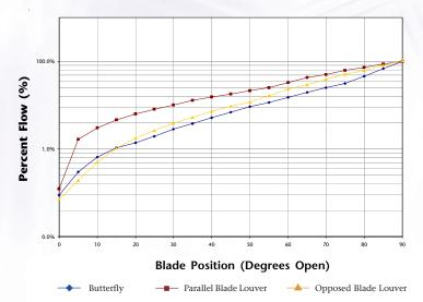
This curve illustrates the advantages of opposed blade dampers and butterflies for fine flow control. These produce nearlinear flow control characteristics as a function of blade position making them ideal for use with positioning devices. Parallel blade dampers provide acceptable flow control exceeding 20-30% full flow. Turbulence produced by parallel blade dampers must be accounted for in the design of duct systems
