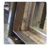
Because there are no seal cavities, there is no area to collect ash and sludge deposits, and corrosion attack of the metallic seals is mitigated.
