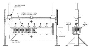
Pathway has performed extensive high temperature cycle testing which has resulted in the development of proprietary design and manufacturing processes. Above is a test fixture which was developed for a major Engineering firm to perform analysis on 800H bellows operating at high temperatures.
