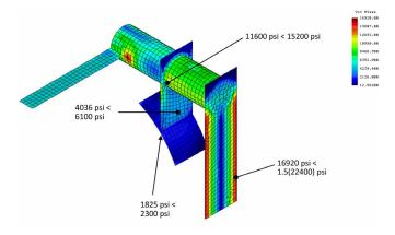
Shown here is an FEA model for the floating torsion pipe design. The floating torsion pipe is not directly welded to the outside of the line pipe to prevent the very high thermal stresses that would result from such an attachment. The torsion pipe and hinge/gimbal hardware is positioned outside of the insulation so that it operates well below the material creep range.
